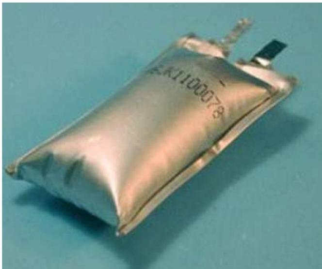
The result of the overcharge is damage to the cells.
